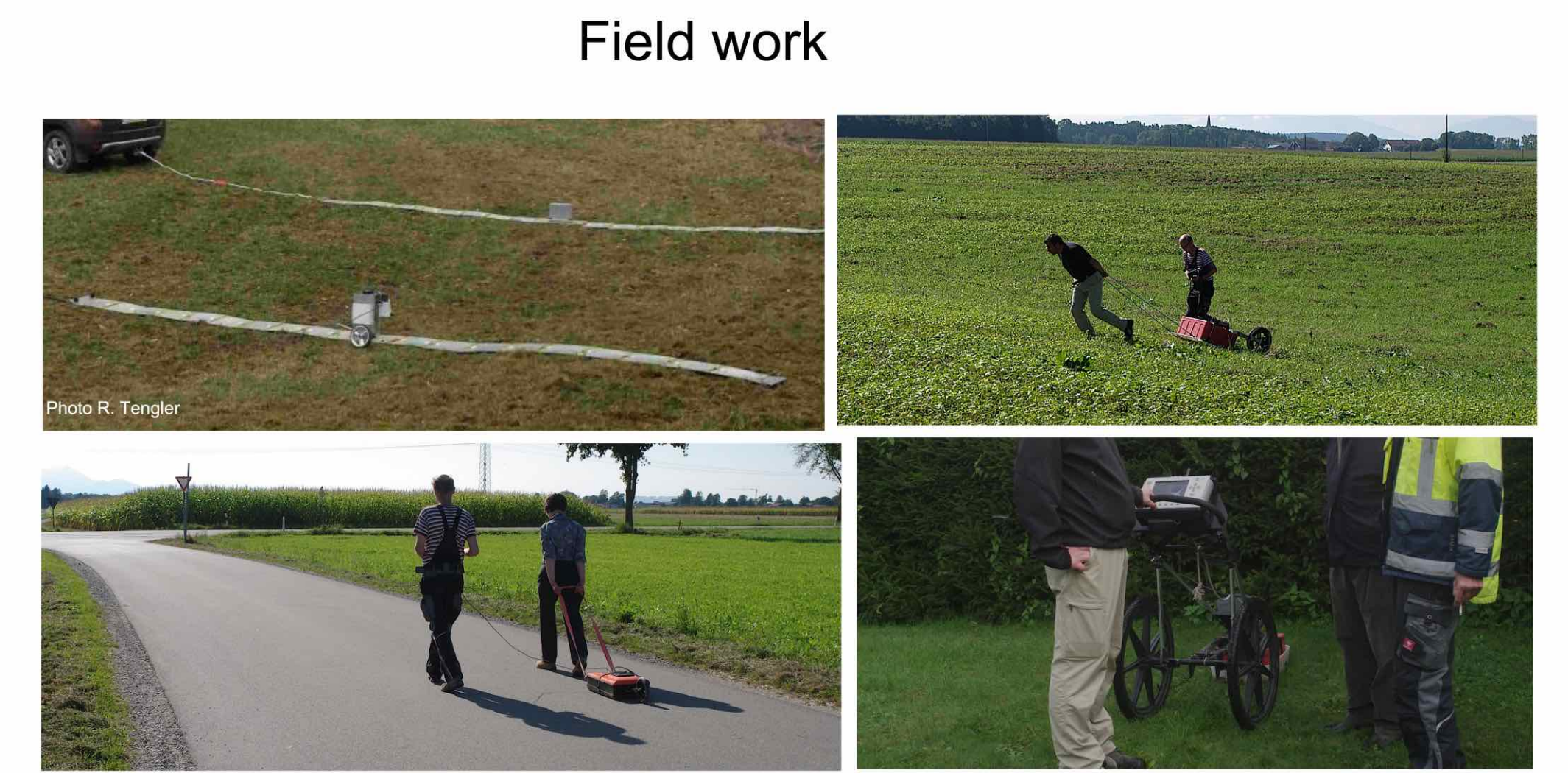
Used GPR equipments: bistatic 25 MHz, monostatic 200, 300, 400 MHz.
